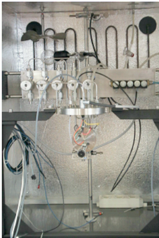
Fig. 2 - The electrolytic cell laid within the thermostated box. The stainless steel UHV containment vessel is missing, thus making electric contacts and the pipes for gases evolved from the electrolysis visible. The electrovalves allowing for automatic gas samples to be sent to the spectrometer for ^4\text{He} analysis are visible in the upper side of the cell
